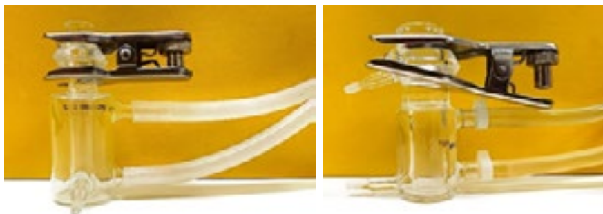
Figure 2. Franz diffusion cell with a volume of 5 mL (left) and 15 mL (right).
