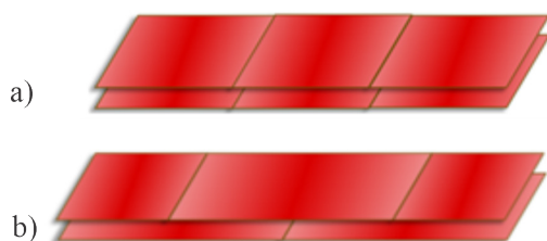
Fig. 4. Schematic diagram of the scanning mode of processing grid superposition; a) repeated scanning of a single grid, and b) cross-stacked scanning of A-B grid
