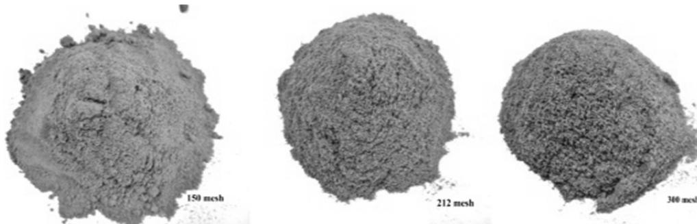
Fig. 1 Teak wood dust of three sizes: 150  $\mu\text{m}$  (left), 212  $\mu\text{m}$  (center), and 300  $\mu\text{m}$  (right)
