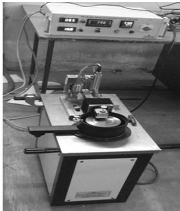
Fig. 5 Friction and wear monitor [20]
