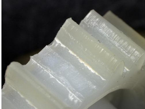
Figure 10: Fatigue of the tooth for POM/PA6 combination after 16.000.000 cycles.
