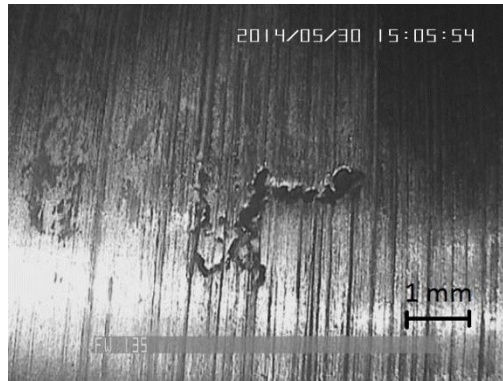
Figure 2. Corrosion damage on inner wall of the tube.
