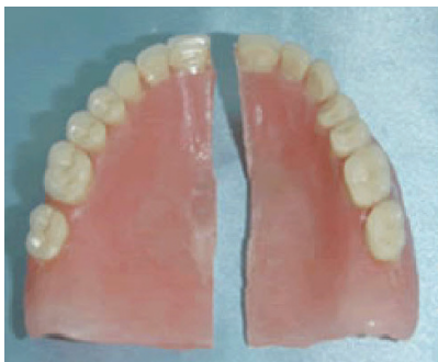
Fig. 1. The midline fracture of complete denture base
