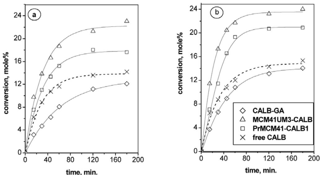
Figure 6. Conversion vs. time in the following reactions: EA + 1-BuOH (a) and EA + 1-HxOH; reaction conditions: 40 °C, 50 mg biocatalyst; EA:alcohol = 3.3:1 (molar ratio); solvent: hexane.
