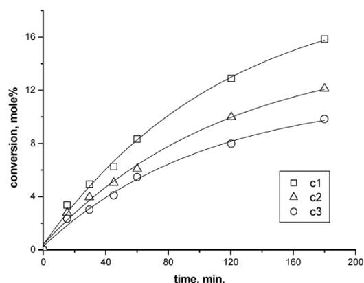
**Figure 7.** Conversion vs. time for PrMCM41-CALB1 catalysed EA + 1-BuOH alcoholysis after 3 catalytic cycles;  $c_i$  ( $i = 1-3$ ) is number of catalytic cycles. Reaction conditions: 40 °C, 50 mg biocatalyst; EA : alcohol = 3.3 : 1 (molar ratio); solvent: hexane.
