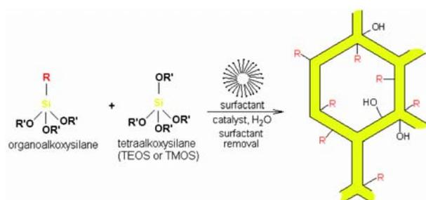
**Figure 2.** Mesoporous silicates functionalization by co – condensation method.
