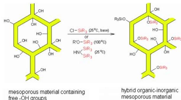
**Figure 1.** Mesoporous silicates functionalization by post-synthesis method.
