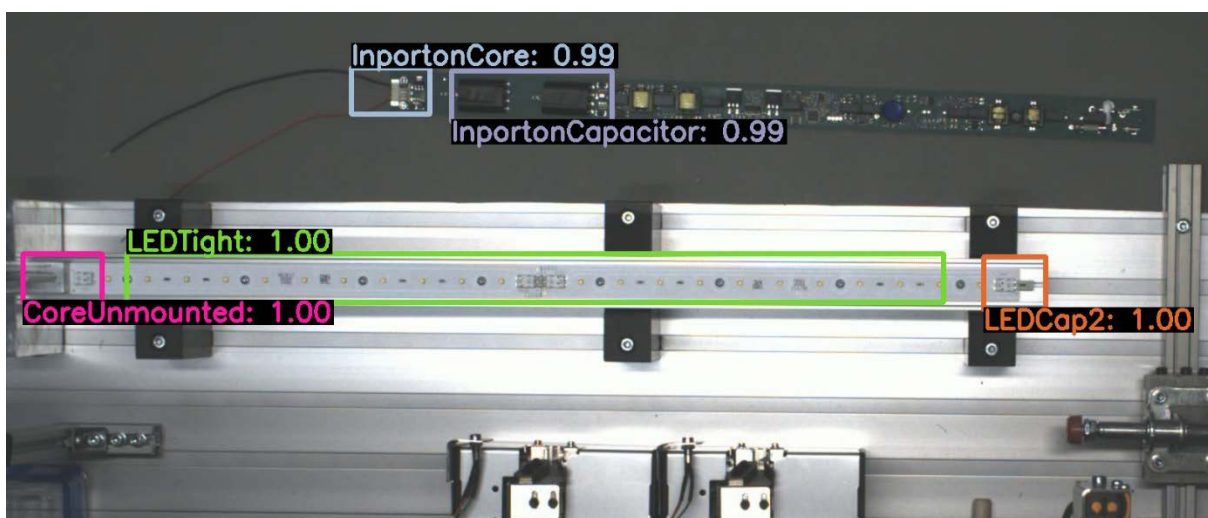
Fig. 2 Inference of a single frame by the trained YOLOv4 model. The inference results are published via MQTT and the corresponding work step or assembly faults are derived based on the detected objects.
