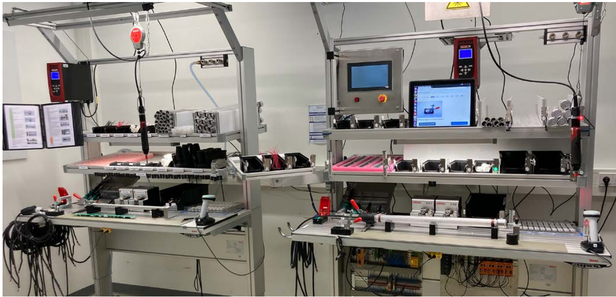
Fig. 3 The workstation on the left is set up without the proposed assistance system and relies on the paper based work instruction on the far left of the picture. The workstation on the right side is equipped with a pick-by-light system and a work instruction visualization. Those are operated with the data supplied by the object detection unit.
