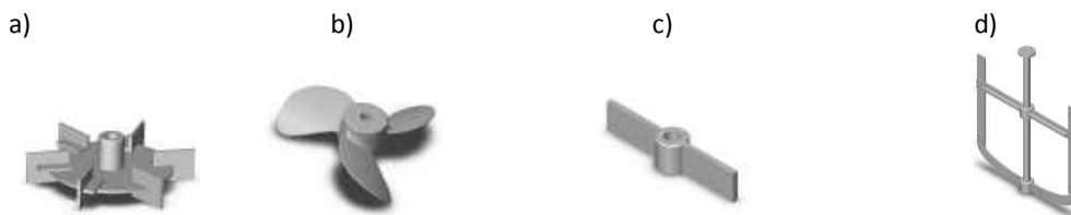
Slika 1.1. Mešala: a) Rushtonova turbina, b) propeler, c) veslo, d) sidro ( http://www.postmixing.com/mixing%20forum/impellers/rt.htm )
