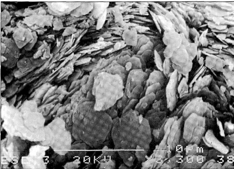
Fig. 4 - Plate like lamellae of hydromagnesite (SEM)
