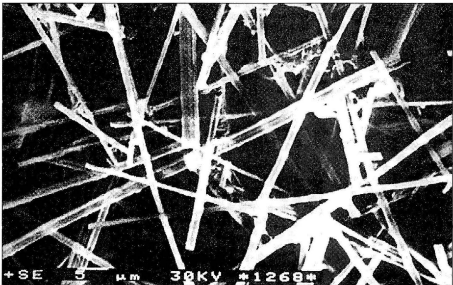
Fig. 1 - Threadshaped calcite crystals (SEM)
