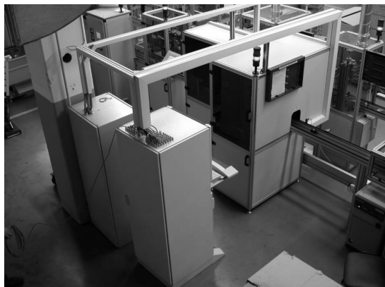
Sl. 2. Diagnostični sistem za sesalne enote Fig. 2. End-quality assessment system installed on the assembly line
