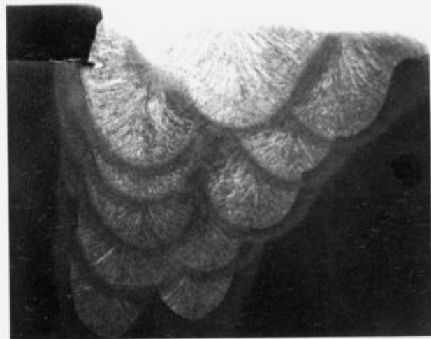
Figure 1: SA weld cross section
