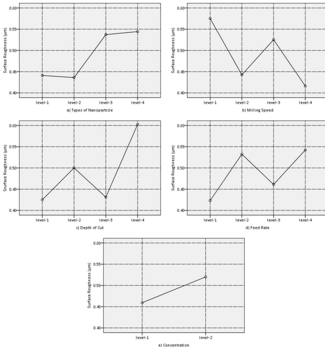
Fig. 5 The surface roughness and related factors with different levels
