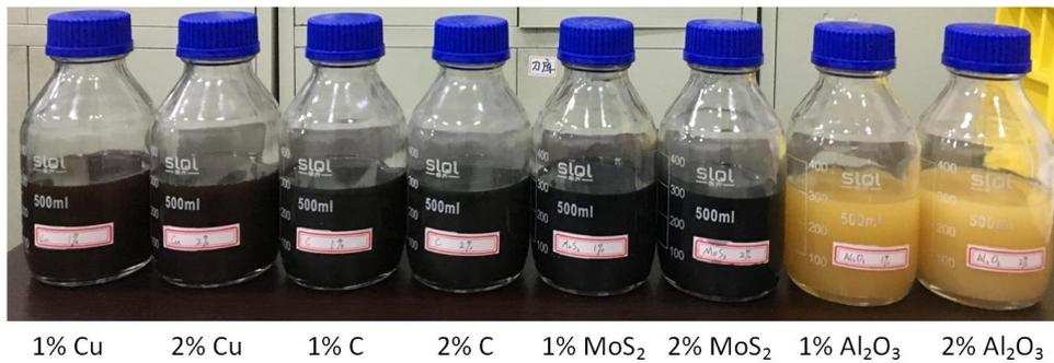
Fig. 1 Nanofluids used in machining process
