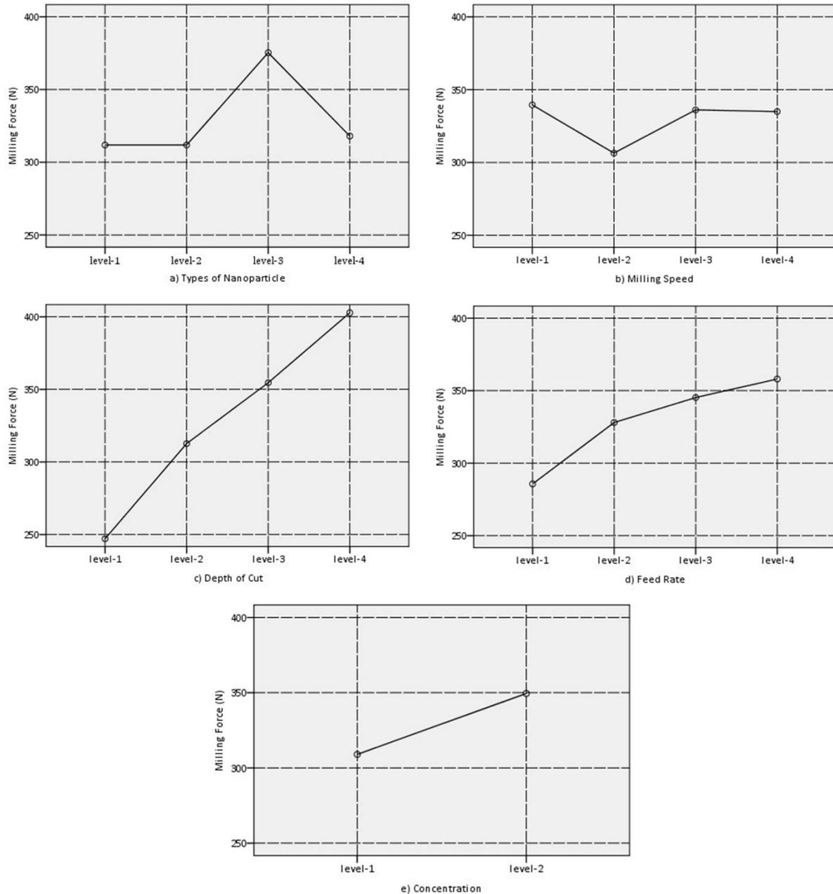
**Fig. 3** The milling force and related factors with different levels
