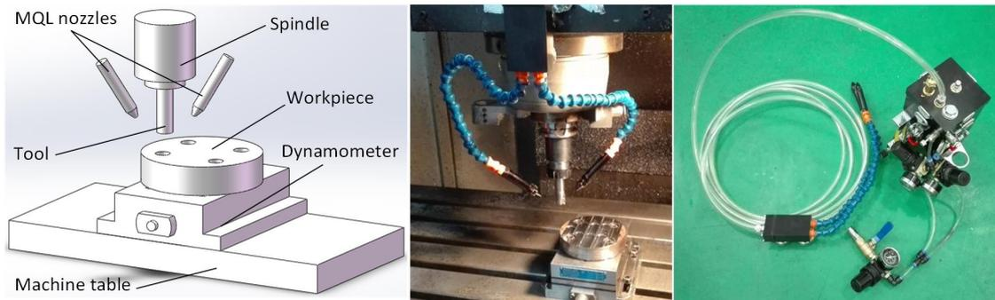
Fig. 2 Experimental setup, machining spot and the MQL device
