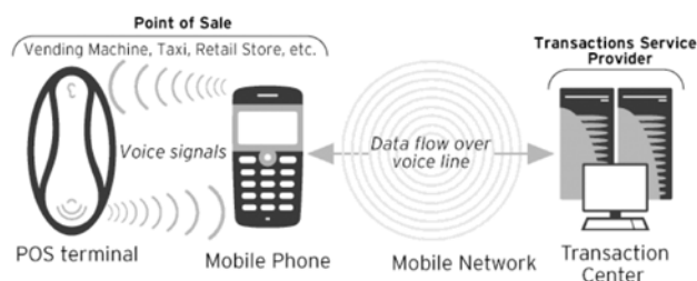
Fig 1: The basic principle of system operation.
