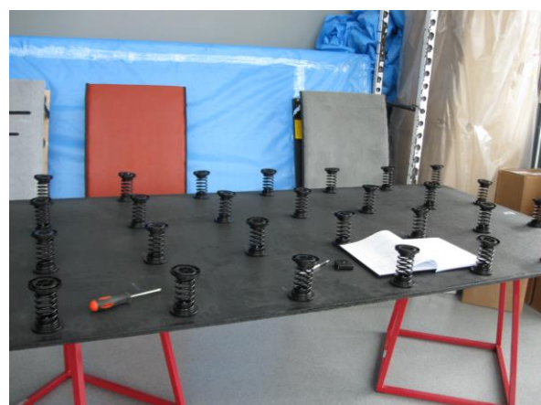
Figure 4. Spring arrangement on the underside of the spring strip panel.
