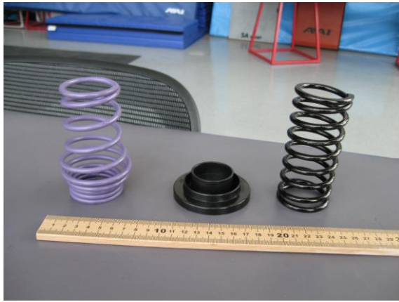
Figure 5. Modified spring on the left, spring end cap in the middle, and an cylindrical spring on the right.
