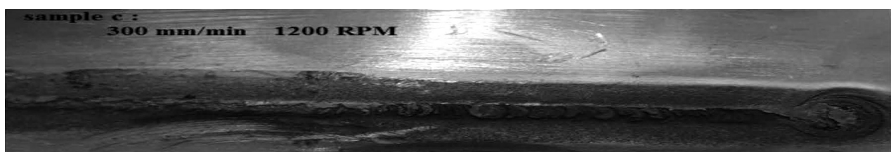
Figure 6: The root of sample C produced at a rotational speed of 1200 \text{ min}^{-1} and travel rate of 300 mm/min
