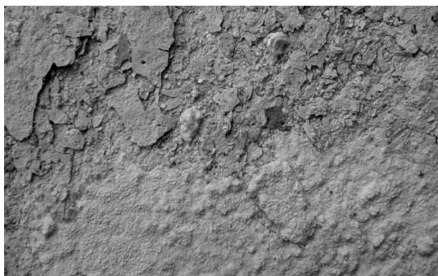
Figure 4: A 6-month exposure to the test environment caused the degradation of the coating based on copolymer acrylate
