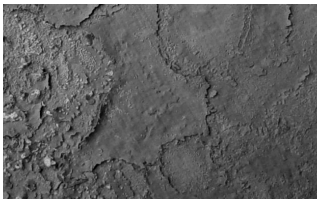
Figure 3: View of the macrostructure of coating based on acrylate copolymer after a 6-month exposure to the test environment
