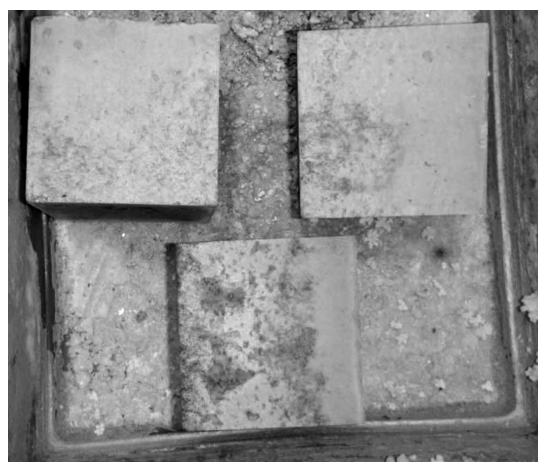
Figure 5: A 6-month exposure to the test environment caused a massive degradation of surface layers of uncoated concrete
