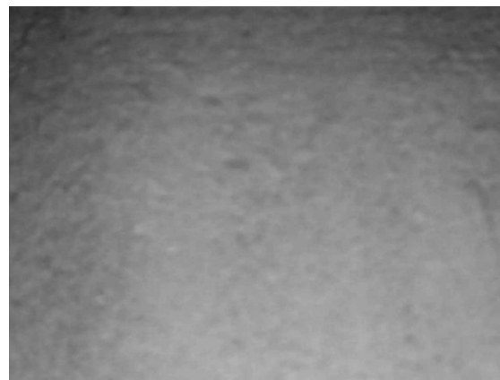
Figure 2: Macroscopic view of the structure of developed AMM coating after a 6-month exposure to ammonium sulphate
