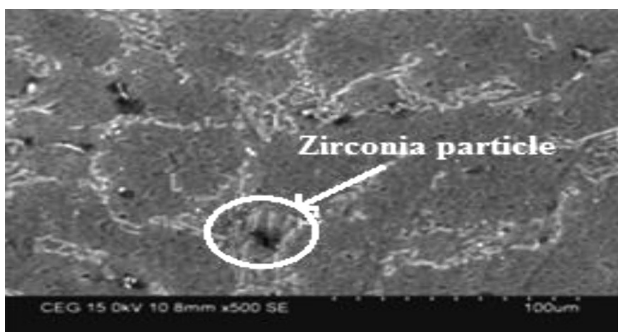
Figure 7: SEM image of LM6–6% of ZrO 2 Slika 7: SEM-posnetek LM6 – 6 % ZrO 2
