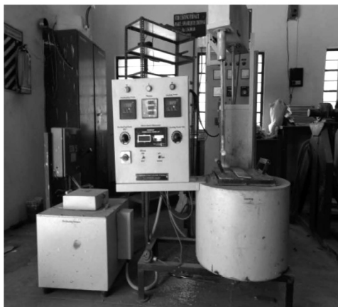
Figure 1: a) Schematic view of stir casting setup, casting of MMC by using stir casting method, b) image of stir casting setup, casting of MMC using the stir casting method
