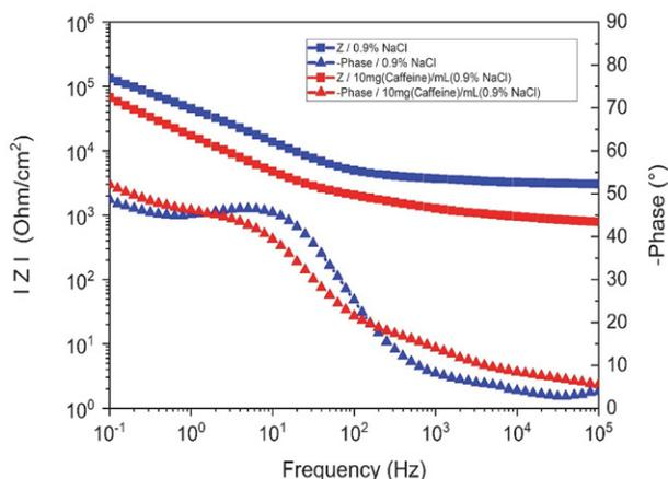
**Figure 4:** Bode diagram of the EIS measurement of the biosensor containing *Saccharomyces cerevisiae* on the WE, with the addition of 0.9% NaCl (blue) and 10 mg Caffeine in 1 mL 0.9% NaCl (red). The Bode diagram includes an impedance diagram described with squares and a phase diagram described with triangles, where  $|Z|$  represents an impedance and  $-Phase$  presents a negative phase shift.
