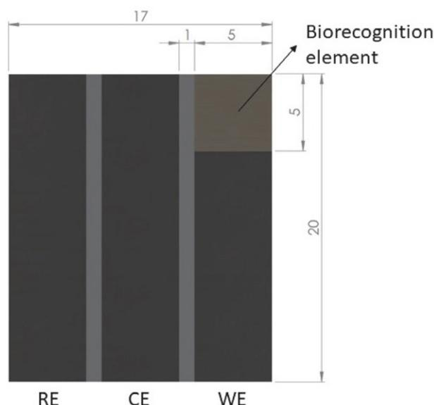
Figure 2: Electrochemical cell in the RCW-side-by-side configuration and the *Saccharomyces cerevisiae* cells attached to the working electrode (WE).
