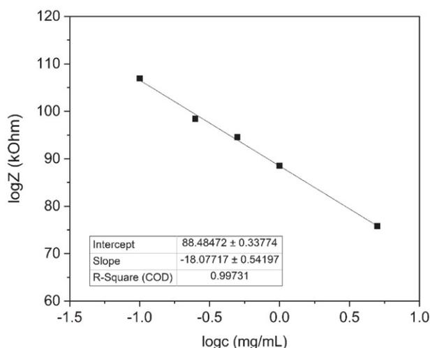
**Figure 7:** Calibration curve between the impedance ( $\log|Z|$ ) and the caffeine concentrations ( $\log c$ )
