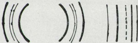
5. sl. Röntgenski posnetek vzorca A montmorillonitne gline iz Cikave Fig. 5. X-ray diffraction of the montmorillonite clay from Cikava A.
