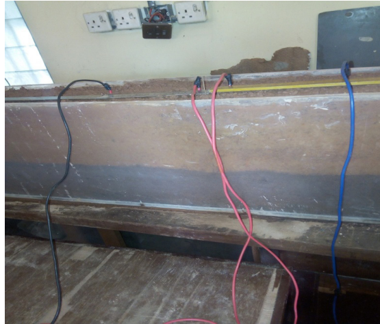
Figure 4: The laboratory setup of three soil layers in a container.
