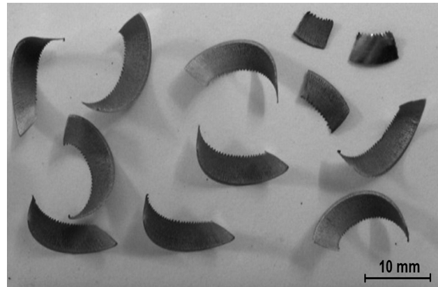
Figure 8: Chip formation at V = 90 m/min
