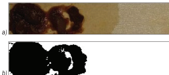
Fig. 5. Before and after the gray processing of residual dirt area by image analysis software; a) before the grey processing of residual dirt area; b) after the grey processing of residual dirt area
