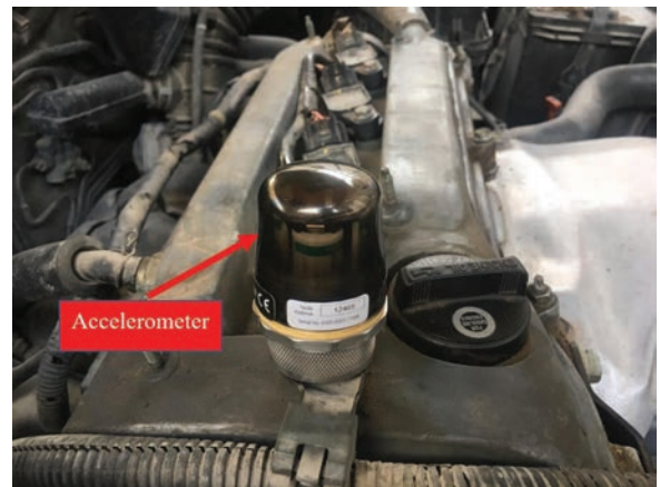
Fig. 3. Mounting of the accelerometer over the engine block
