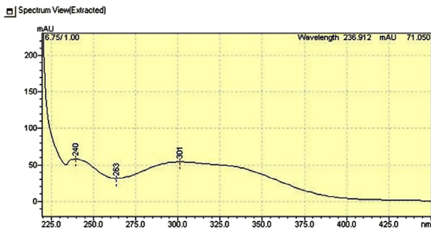
Figure 2. Absorption spectra of nimesulide (maxima at 240 nm and 301 nm)
