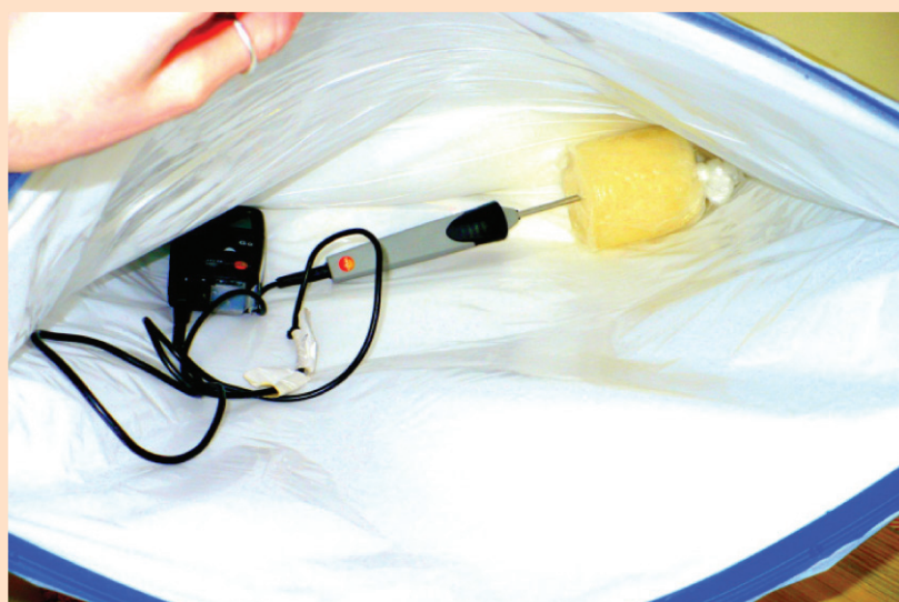
Picture 2: Test product together with the data logger and thermometer probe in the insulating bag
