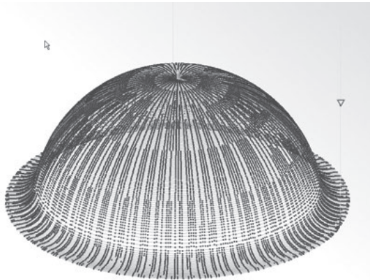
Fig. 12. NC program simulation of toolpath 3
