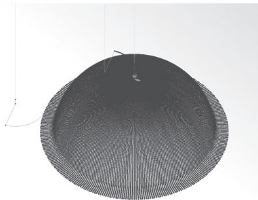
Fig. 14. NC program simulation of toolpath 4
