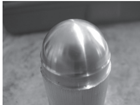
Fig. 19. Finished part after toolpath2
