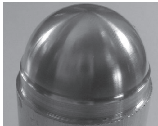
Fig. 23. Finished part after toolpath 4
