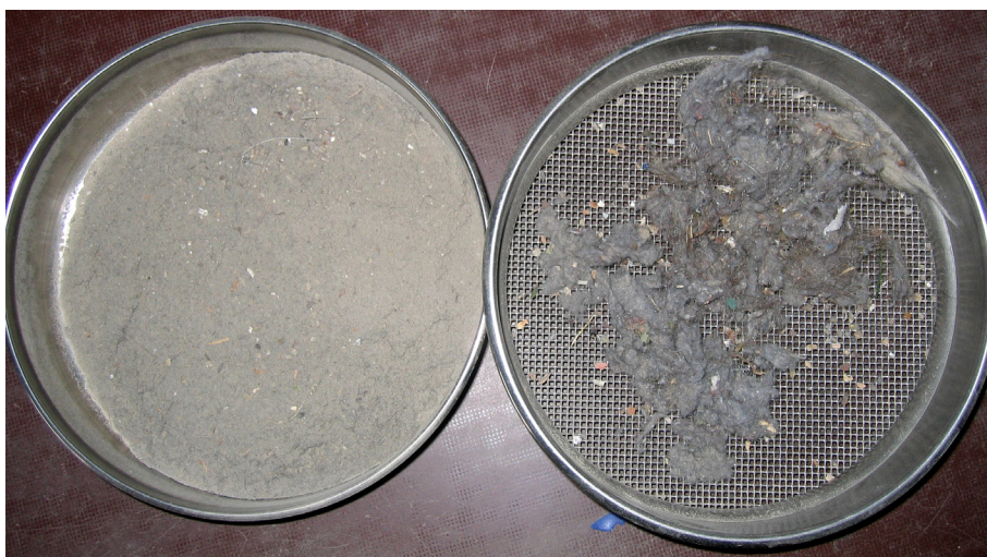
Fig. 4. Household dust preparation. Material was rubbed on the 1 mm sieve. Fibres (right) were discarded, remains (left) were sieved several times on 0.5 and 0.125 mm sieves to remove as much smaller fibres as possible.
