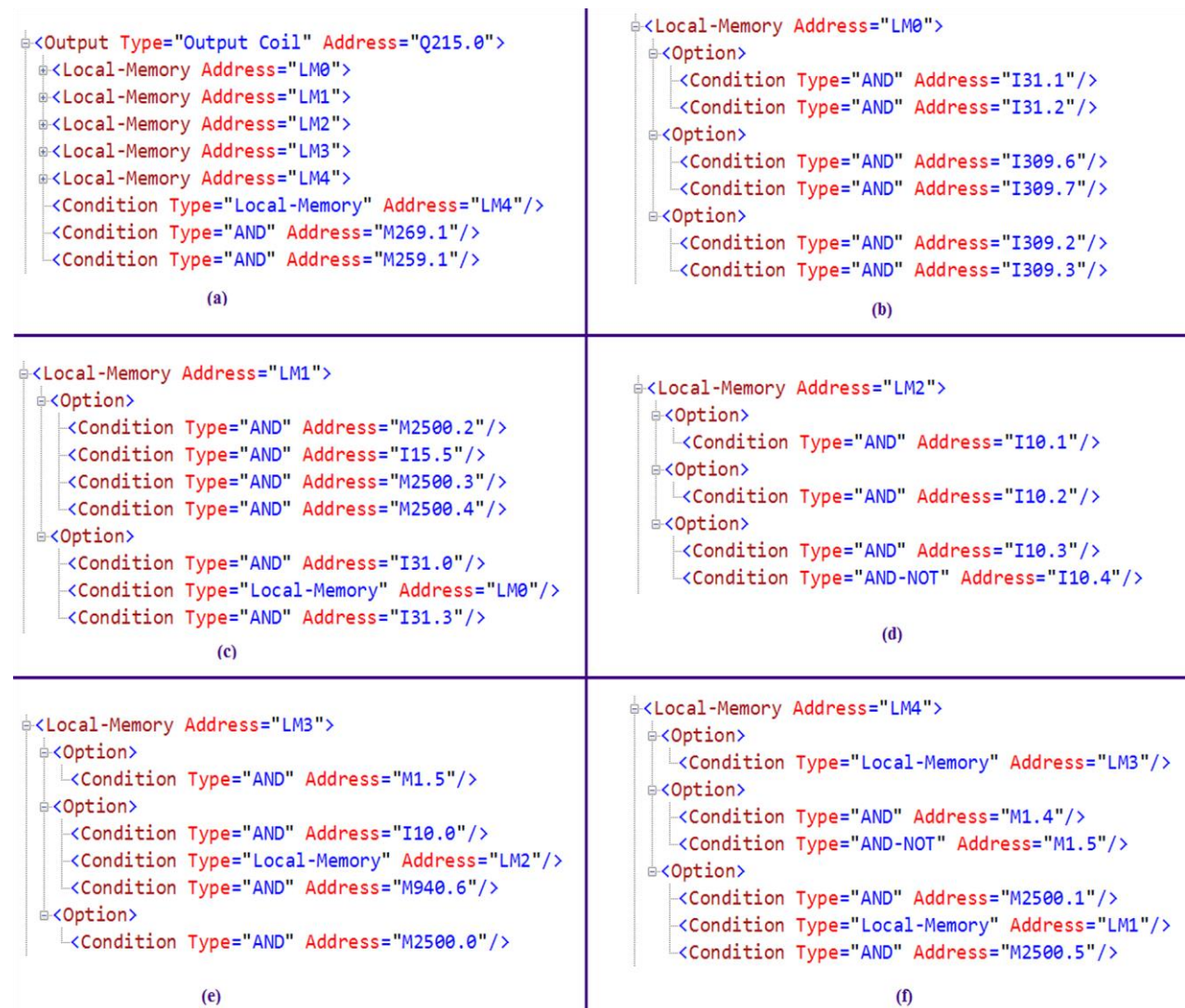
Figure 6: XML file format for the rung diagrams with parallel branches and sub-branches. (a) The condition set corresponding to the first Output Coil instruction. (b) Local memory LM0 definition. (c) Local memory LM1 definition. (d) Local memory LM2 definition. (e) Local memory LM3 definition. (f) Local memory LM4 definition.
