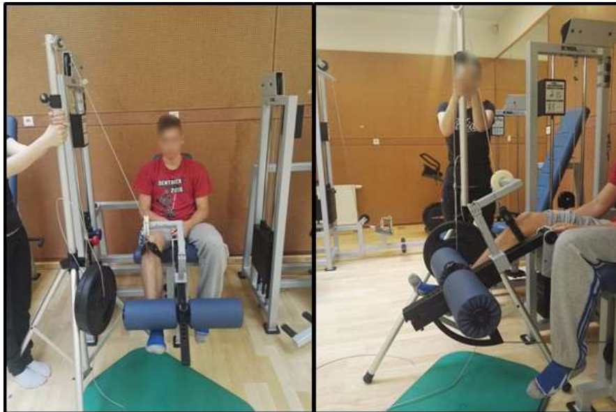
Figure 1. The machine with self-standing stand and the part fixed on the seated knee extensor training device for coupling active and passive loading of the knee.
