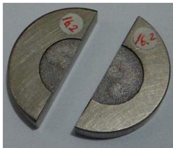
Fig. 3. A machined Ti-6Al-4V workpiece
