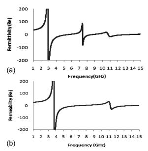
**Figure 3:** a) Real magnitude of permittivity ( $\varepsilon$ ) against frequency, b) real magnitude of permeability ( $\mu$ ) versus frequency **Slika 3:** a) Realna magnituda permitivnosti ( $\varepsilon$ ) proti frekvenci, b) realna magnituda permeabilnosti ( $\mu$ ) v odvisnosti od frekvence
