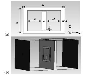
Figure 1: a) Design of the unit cell, b) simulation geometry in CST software
