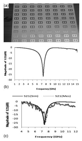
**Figure 2:** a) Prototypes for measurement, b) simulated transmission coefficient  $(S_{21})$  for *z*-axis wave propagation, c) comparision of measured and simulated result for  $S_{21}$
