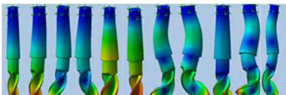
Fig. 19. Mode shapes of a tool without a heat pipe
