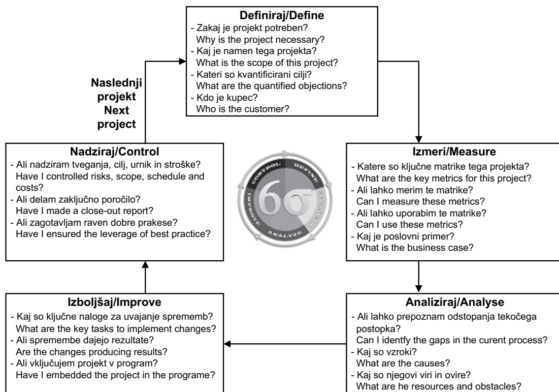
Sl. 6. Krog DMAIC kot osnova metodologije Šest Sigma Fig. 6. The DMAIC cycle as a methodology for Six Sigma
