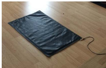
Figure 3. Fitro Jump ergometer (Zemkova & Hamar, 2004).
