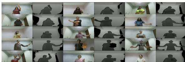
Figure 5: Our Dynamic Hand Gesture Dataset. Microsoft Kinect is used to capture the gestures of 5 users in RGB and depth modality. There are 16 gestures classes, 10 of which were taken from Jacob et al. [14], and a no system action class. Sequences are recorded with 3 varying backgrounds (blue, green and pink) and 3 different scales (user distance from the camera - 1, 2, 3 steps from the camera) performed each on their left and right hand unless the gesture needs two hands to perform. For each take, the users were asked to dress differently and apply different hairdos to increase variability. The dataset includes 1400+ gesture samples.
