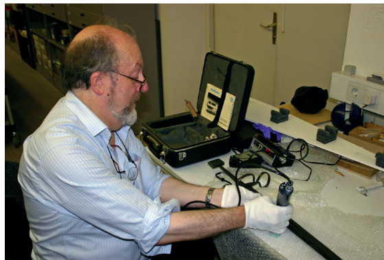
Figure 11: Investigating a 15th century sword blade with a portable hardness tester. (Photo: T. Lazar)
