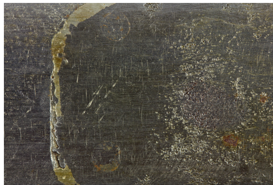
Figure 1: Macro photograph of an old repair – details of riveting and brazing on a 16th century sword blade. (Photo: T. Lazar)
