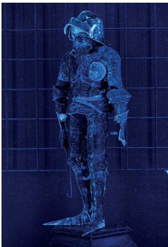
Figure 3: UV photography of a miniature suit of armour easily identifies various layers of varnish. (Photo: Andrej Hirci)
