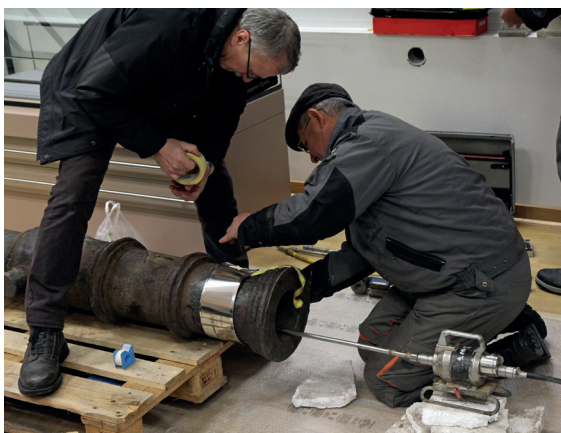
Figure 7: Preparation for Ir-radiography of a late medieval cannon. (Photo: T. Lazar)
