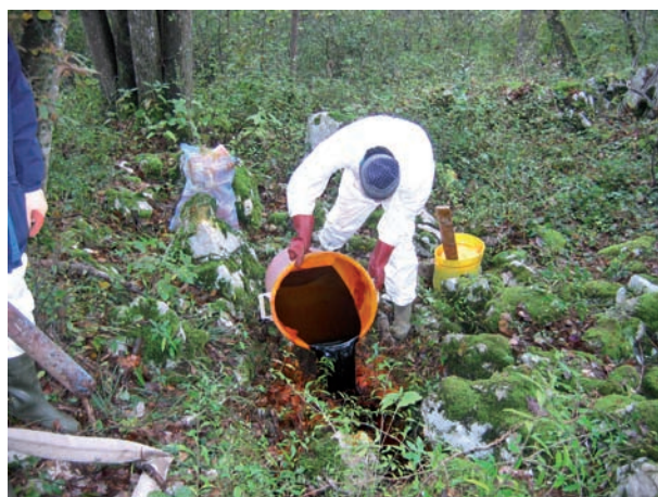
Fig. 5. A solution of uranine was injected into a well permeable fissure at the margin of the landfill.
