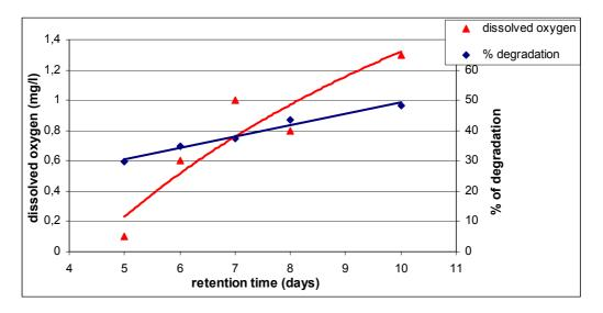
Figure 10 – dissolved oxygen and % of degradation in aerobic digestion as a function of HRT
