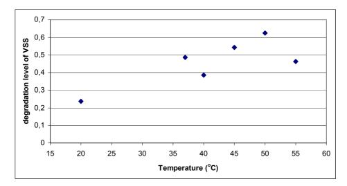
Figure 6 – Temperature dependence of aerobic degradation (cross-section of Figure 5 at 17 days as a function of temperature)
