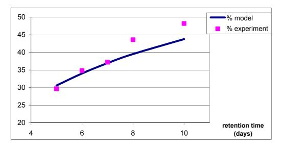
Figure 9 - Degradation levels of aerobic digestion: model and experiment
