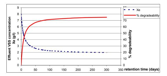
Figure 8 – Model for continuous aerobic digestion
