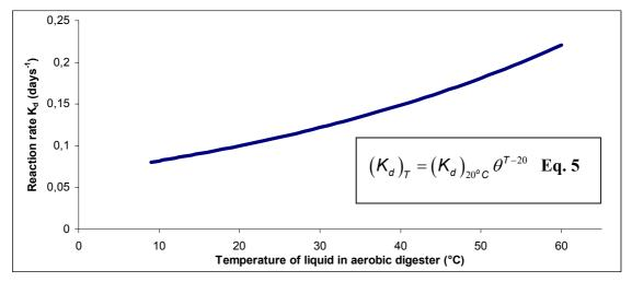
Figure 1 – Aerobic digestion reaction rate as a function of temperature
