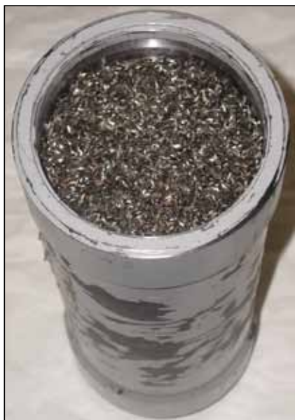
Figure 9. Prototype of gas bottle with regenerative heat exchanger made out of steel cutting
