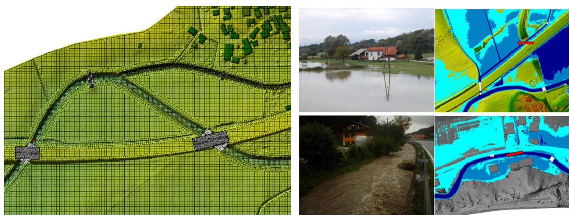
Figure 8. Hydraulic model mesh (left) and validation results (right)
