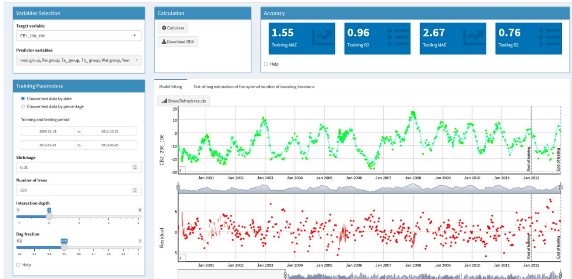
Figure 2. Interface of SOLDIER during model fitting. Target and input variable selection (top left), training period and model parameters (bottom left), accuracy measures for training and test (top right) and graphical representation of predictions, observations and residuals (bottom right)
