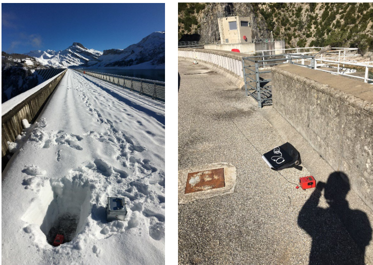
Figure 3. Position of the recording device on the crest of dams
