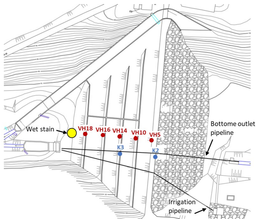
Figure 3. (a) Layout plan of the dam with appurtenant structures; (b) location of the geodetic points VH5, VH10, VH14 and VH16; (c) location of the piezometers K2 and K3; and (d) location of the wet stain.
