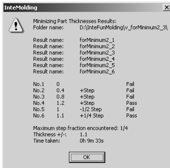
Fig. 10. Thickness minimization results after the changed molding-quality criteria
