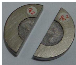
Fig. 3. A machined Ti-6Al-4V workpiece
