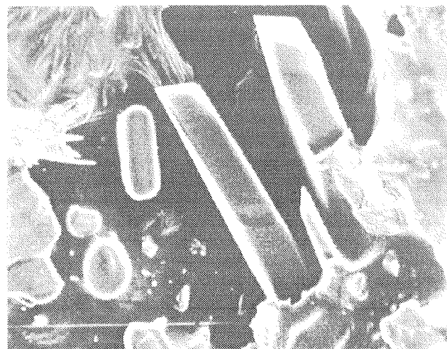
Fig.9: Formation of crystalline structure after cooking and drying of polyamid particles (SEM, magn. 800)
