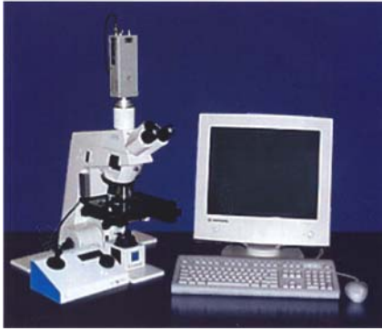
Fig. 1. A computerized stereology system (Stereologer, Systems Planning and Analysis, Inc., Alexandria, VA).
