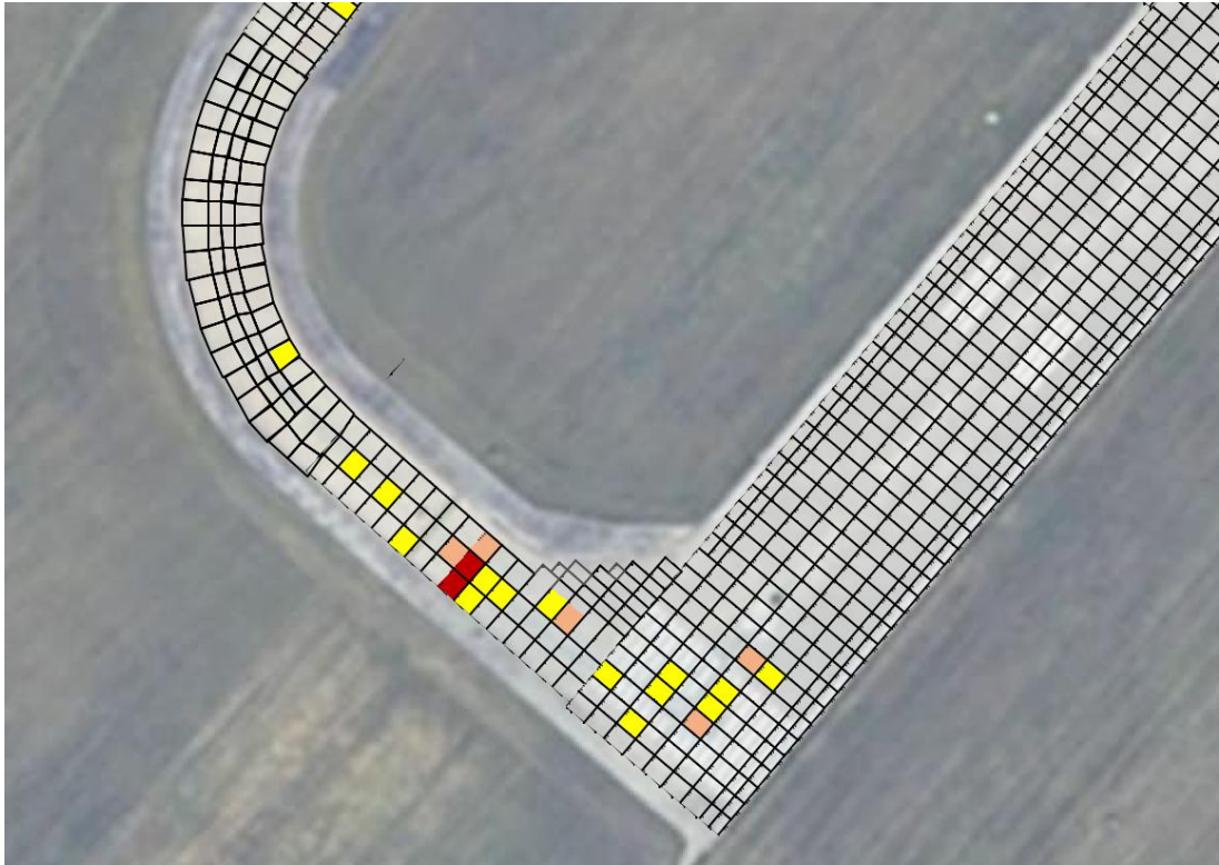
Figure 1: Broken slab corner defect occurrence map.
