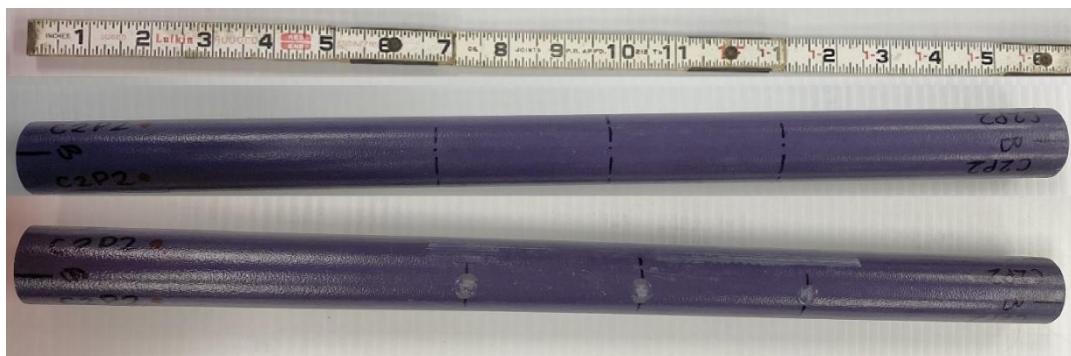
Figure 4: Partial coating failure due to impact testing.
