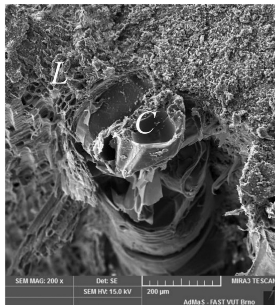
Figure 9: SEM micrograph of adhesive failure for FRP/oak, existence of the adhesive in the lumina of vessels (V) and libriform (L), magn. 200×
