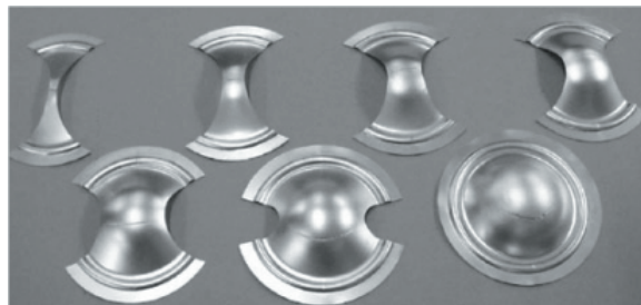
Fig. 8. Nakajima test specimen geometries
