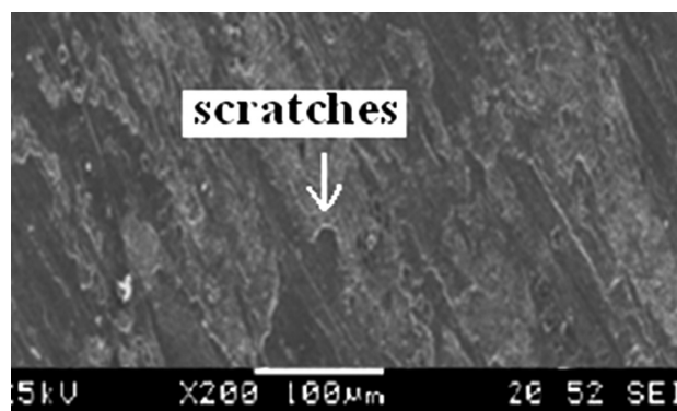
Figure 11: SEM micrograph of the worn surface of the AA6061-B 4 C-Gr composite at the normal load of 20 N and 1 m/s sliding velocity
