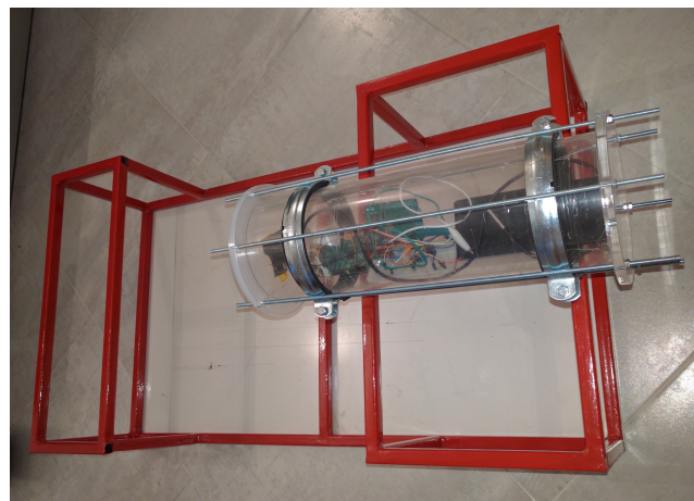
Figure 1. SeaAbs: a low cost seafloor observatory before materials are mounted on
