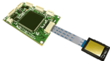
Fig.3. Fingerprint Reader Module (Suprema Technical Manual, 2007)
