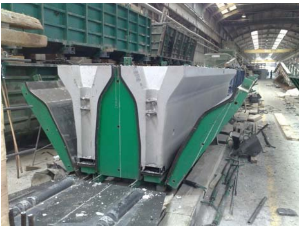
Figure 11: Elements of new Jersey concrete barriers.
