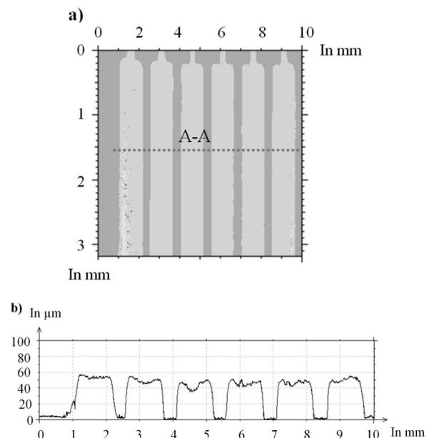
**Figure 3:** a) Image of the six as-deposited elements on Au/Al<sub>2</sub>O<sub>3</sub>. b) Profile of the six as-deposited elements on Au/Al<sub>2</sub>O<sub>3</sub> measured by profilometer.
