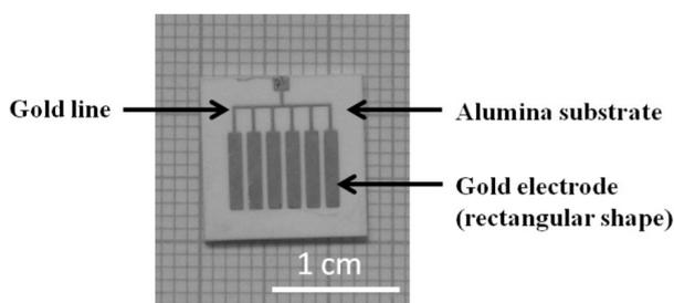
**Figure 1:** Representative  $\text{Au}/\text{Al}_2\text{O}_3$  structure consisting of 6 aligned rectangular gold electrodes with a length of 6 mm, a width of 1 mm and a space between electrodes of 500  $\mu\text{m}$ .
