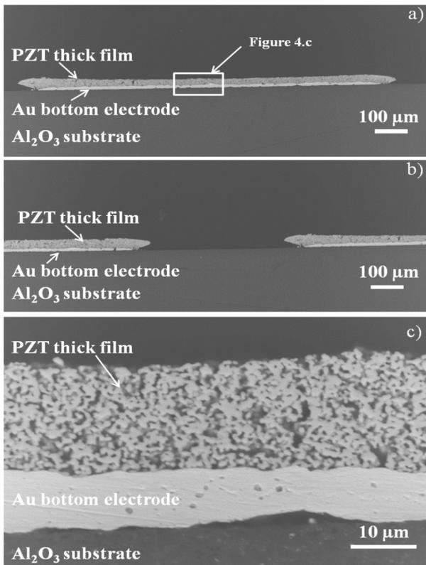
**Figure 4:** PZT-PbO thick films on a flat Au/Al<sub>2</sub>O<sub>3</sub> substrate sintered at 950 °C for 2 h. SEM cross section image of a) one element; b) two elements and kerf in the middle. c) Inset from Figure 1a) (magnification x 2000)
