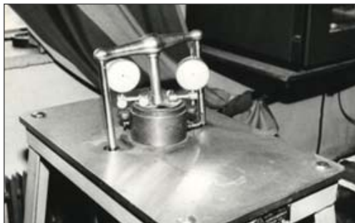
Figure 3. Swelling test in an oedometer under load.
