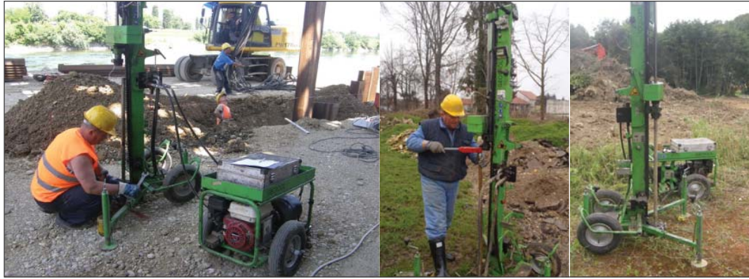
Figure 6. Geotool dynamic probing rig (Dynamic Sampling Ltd, UK). The rig is capable of dynamic probing (DPL-light, DPM-medium, DPH-heavy and DSPH-super heavy) in accordance with DIN 4094. Specification: Width 78 cm, Length 78.5 cm, Height 23.4 cm, Drop Height 50 cm, Rod/Tool Length 120 cm (max) and Basic Weight 125 kg. Reference penetration every 100 mm. Base area of cone 20 cm 2 . Cone diameter 43.7 mm. Rods diameter 32 mm. Hammer mass 50 kg. Drop height 50 cm. Angle of the cone point 90°. Torque wrench for impact of rod skin friction.
